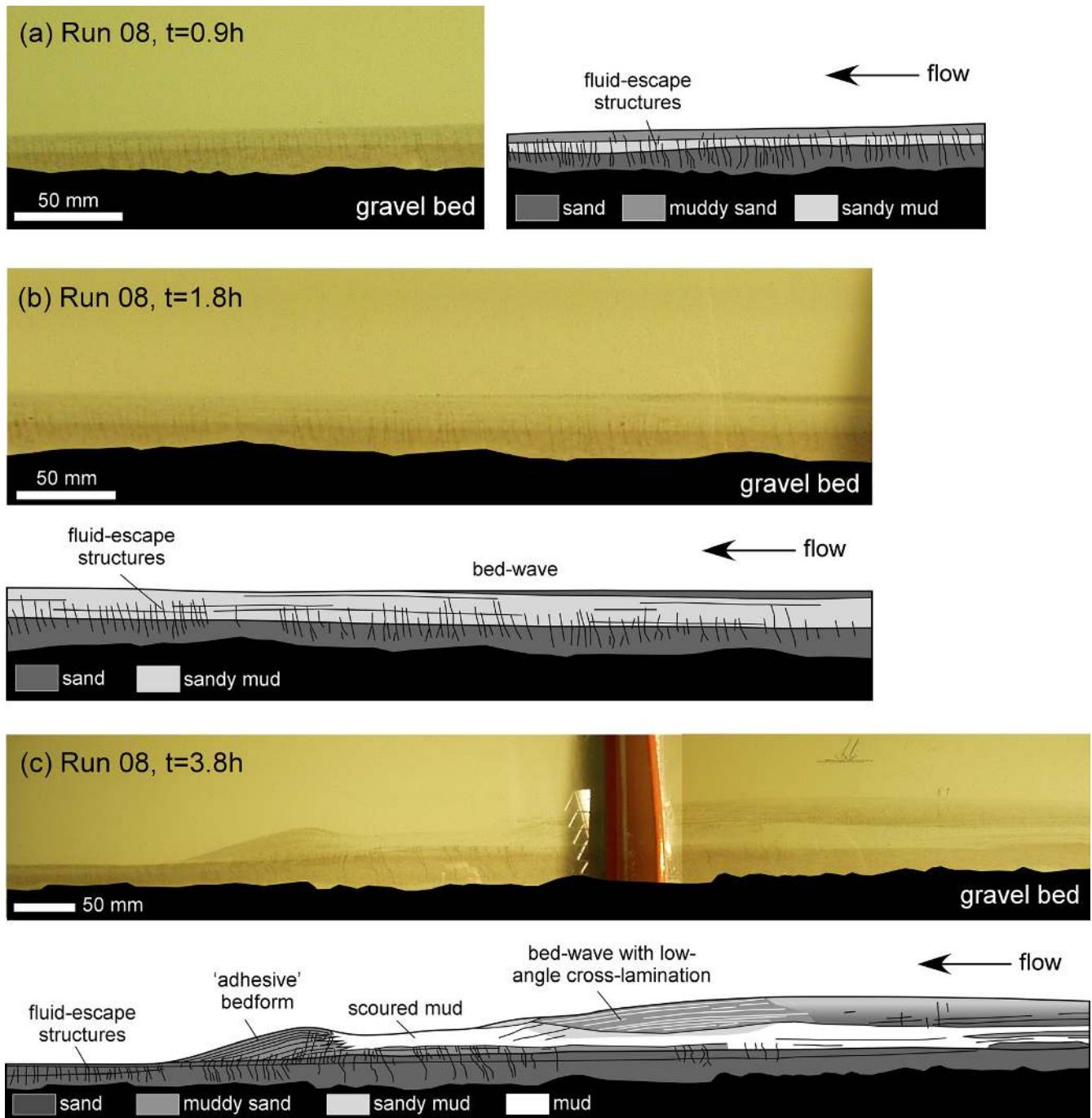
Fig. 21. USPB-equivalent bedforms in the middle stability region of lower transitional plug flow. (a) 0.9 h, (b) 1.8 h, and (c) 3.8 h after the start of Run 08. The scour with complex primary current lamination is notable.
