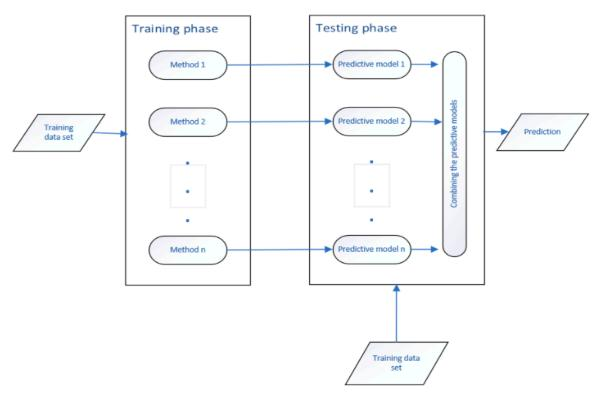
Figure 3. Ensemble method flowchart.
