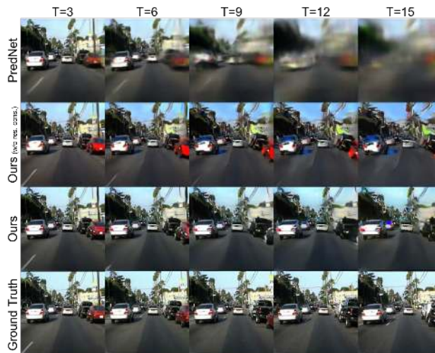
Figure 1. A comparison of predicted frames in a driving environment [5]. The state-of-the-art method, PredNet [17], predicts blurry images as the time step increases, whereas the proposed method shows relatively sharp and accurate images. Here, PredNet uses ten images as input whereas our method takes four images to predict future.
