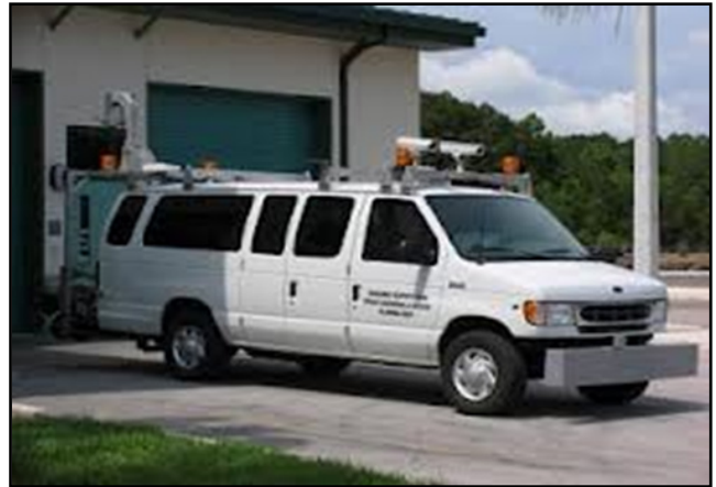
Figure 1. Specialized Van for IRI Data Collection
