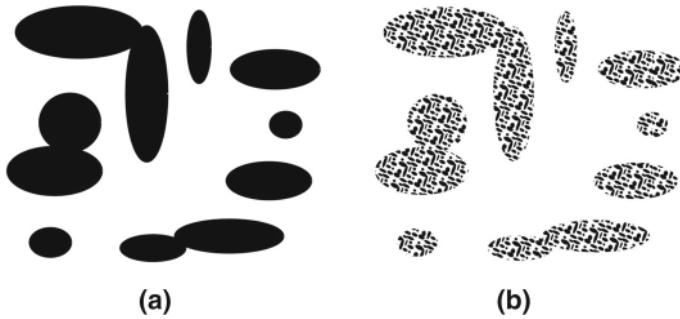
Fig. 2 Example of a connected pore space with grains in black (a). If we replace the dense grains with microporous grains (b), this microporosity will dominate in the evaluation of Minkowski functionals, but it will not change the permeability significantly
