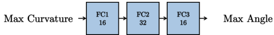
Fig. 7: Network architecture that maps angle from curvature. Each fully-connected (FC) layer is followed by a ReLU activation and batch normalization.
