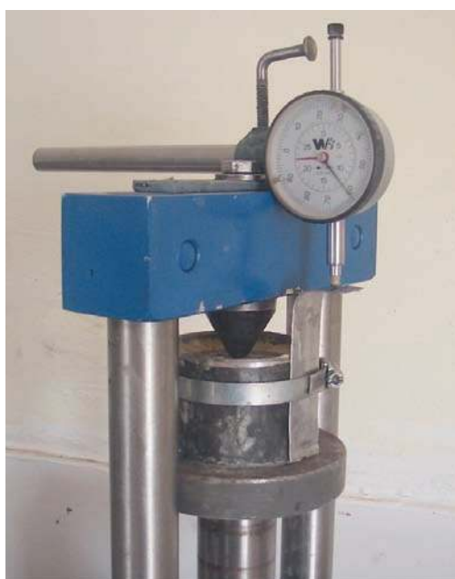
Figure 2—Indentation testing using point load apparatus
