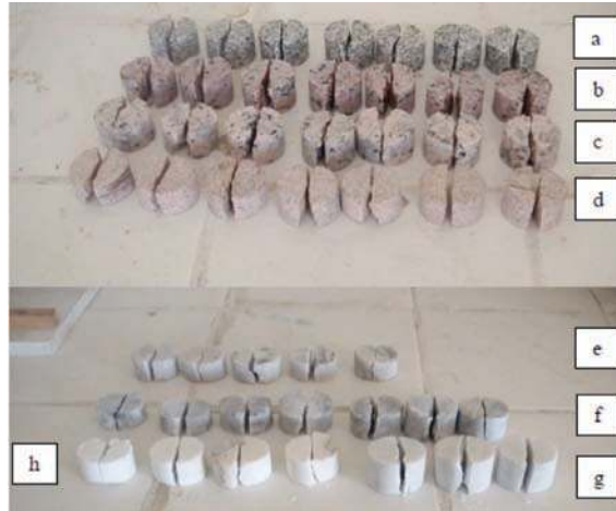
Figure 5—Some samples that failed in the Brazilian tensile test: a) Kozak/Balikesir granite b) unknown granite (King Rosa), c) Kaman/Kirsehir granite (Kaman Rosa), e) Marmara Island/ Istanbul marble, f) Iscehisar/Afyon marble (Kaplan postu), g) Uckapili/Nigde marble, h) Milas/Mugla marble
