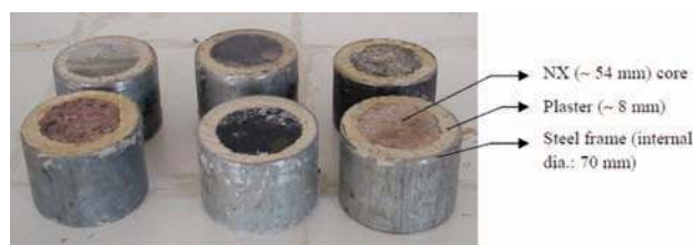
Figure 1—Cemented samples in the circular steel frames
