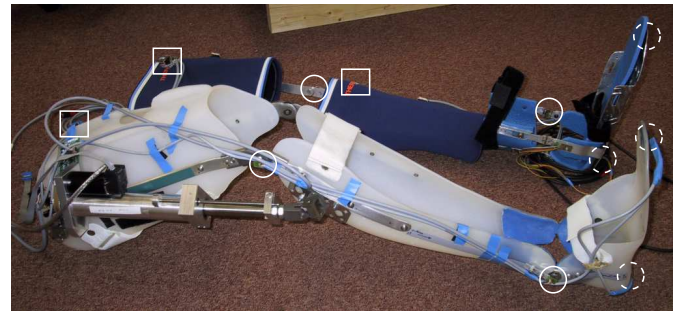
Fig. 1. This image shows the orthosis with the attached actuator and all pose sensors in the foreground (Hall sensors: solid circles, accelerometers: squares, floor contact sensors: dashed circles). In the background the light-weight orthosis for the left leg can be seen.
