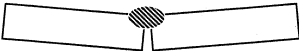
(c) Type 3 distortion caused by Modes 1 and 2 movements and Mode 3 rigid body movements
