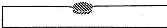
(a) Type 1 distortion that involves only Mode 1 movements caused by plastic deformation produced during welding
