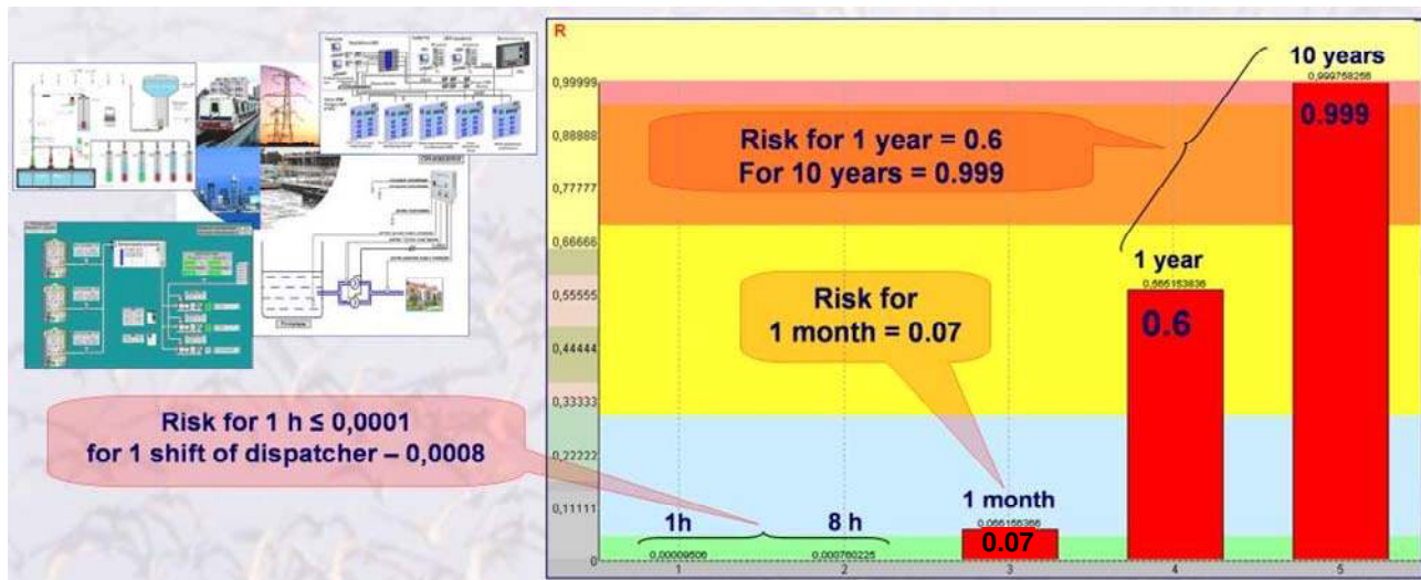
Figure 20. Results of modelling a SCADA-system.
