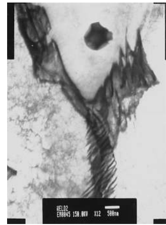
Fig. 11. TEM micro photograph of sample P14 showing acicular ferrite nucleated by inclusion within grain boundary.
