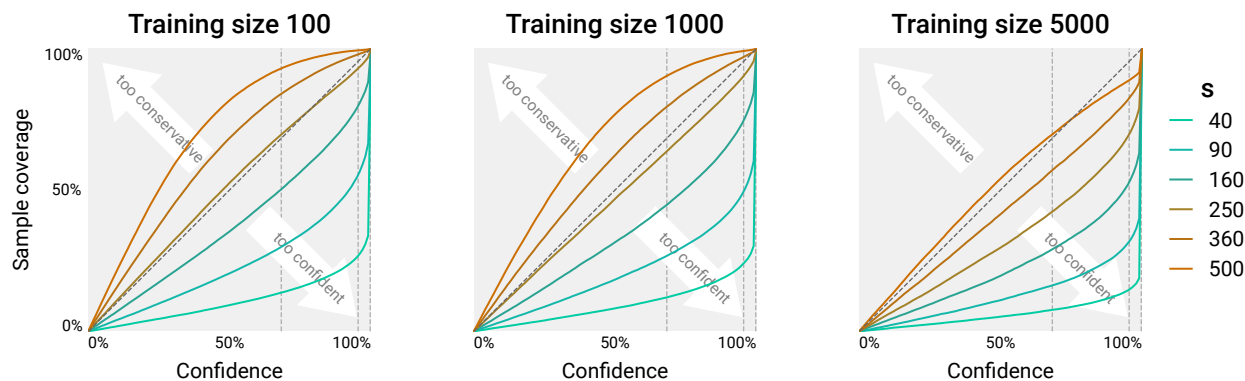
Figure 6: The generalized starting probability parameter s determines the width of the predictive confidence interval, which should contain a proportional percentage of the ground truth energy of the test samples. Smaller s values lead to aggressive confidence interval estimations, yielding coverage curves below the diagonal. Larger s values, in contrast, lead to conservative estimations and wide confidence intervals, yielding curves that lie above the diagonal.
