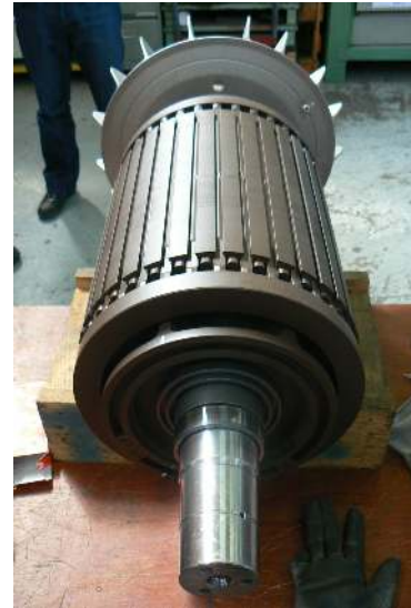
Fig. 11. New rotor of the industrial 250 kW motor.
