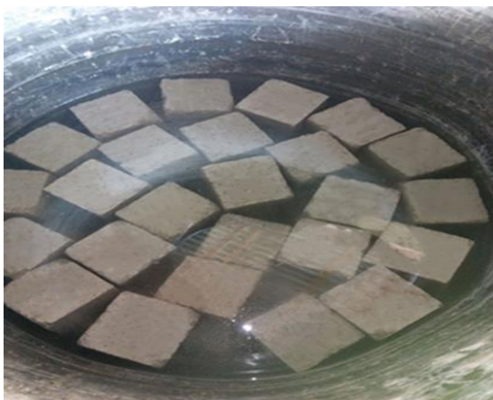
Fig. 5 Curing of Concrete Cubes
