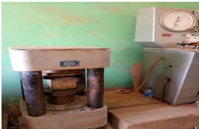
Fig. 3 Destructive Compression Test on Concrete Samples
