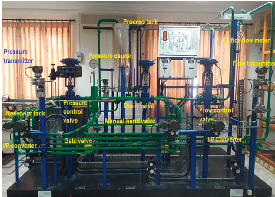
FIGURE 1: Experimental hardware for water distribution system.
