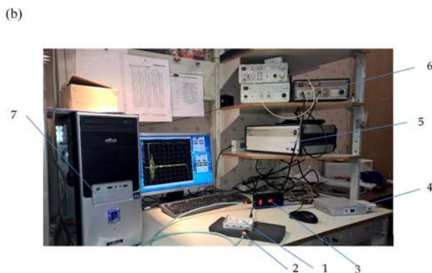
FIGURE 3. A block diagram of an experimental measurement of the delay time of a prototype of the meander microstrip line (a), and a general photograph of the experiment (b); where 1 is the meander delay line-under-test, 2 is the attenuator, 3 is the pulse shaper GZ117GN-03, 4 is the sampling unit SU-3130, 5 is the digital sampling precision converter SD20037, 6 is the pulse generator mainframe GZ-1106DL2, 7 is the computer with the control software.
