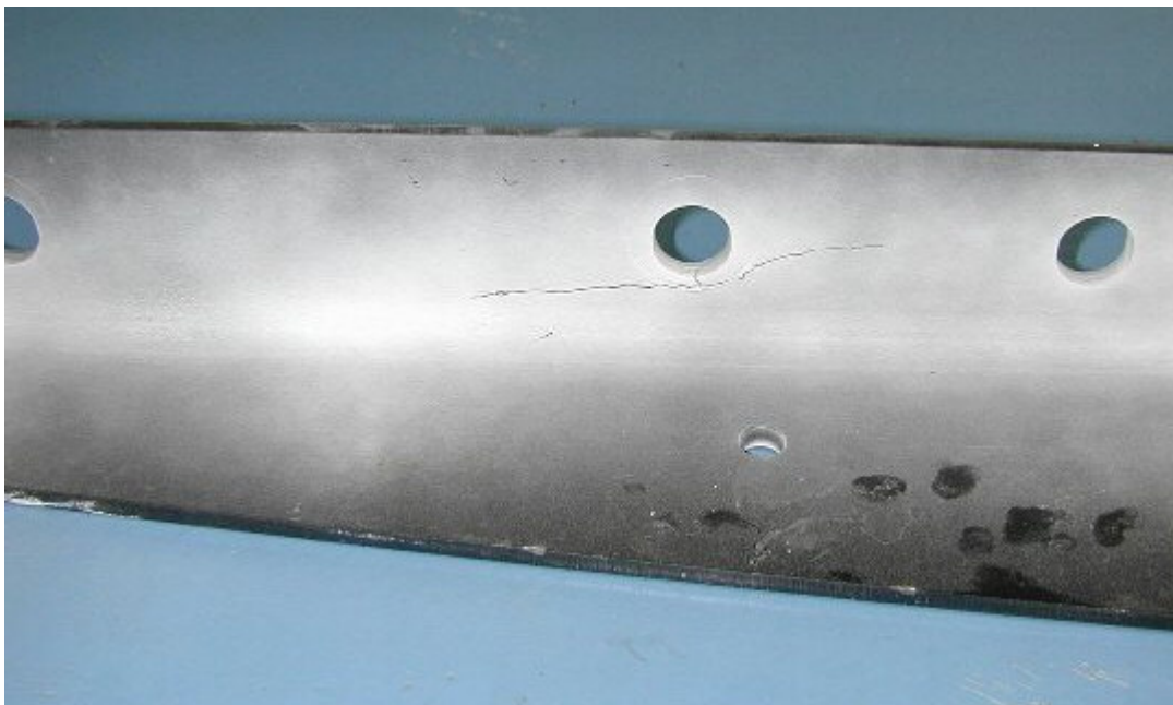
Figure 7: Fatigue failure at the hot-spot during testing
