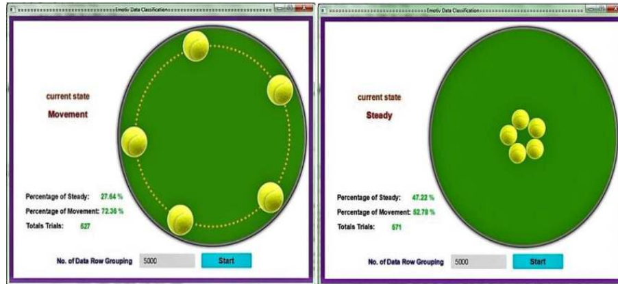
Figure 8: Classify real-time motor imagery tasks via developed brain game, presenting movements and steady correspondingly.
