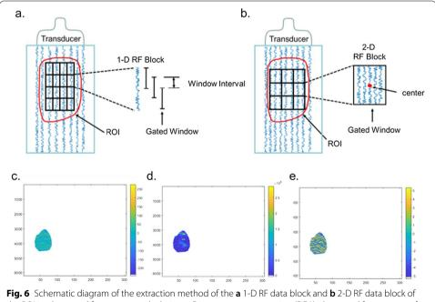
**Fig. 6** Schematic diagram of the extraction method of the **a** 1-D RF data block and **b** 2-D RF data block of the ROI in ultrasound feature map calculation. **c** Direct energy attenuation (DEA) ultrasound feature map. **d** Skewness of spectrum difference (SSD) ultrasound feature map. **e** Noncentrality parameter S of the Rician distribution (NRD) ultrasound feature map
