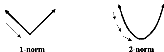
Figure 4. The weights of irrelevant descriptors will converge to zero much faster when using the l_1 -norm compared to the l_2 -norm.
