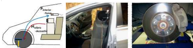
Fig. 9. Experimental set-up for the vibro-acoustic transfer function
