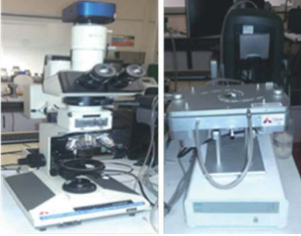
Figure 2 Apparatus used for the coalescence experiment: optical microscopy (left) and hot-stage instrument (right) used for coalescence test.
