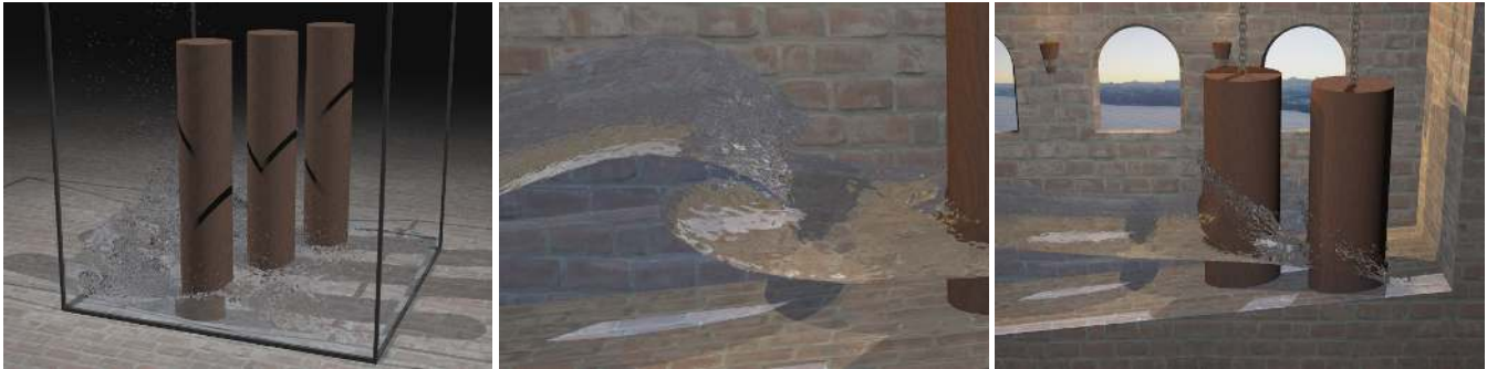
Figure 1: Three examples produced with our incompressible simulation: (Left) 2M particles splashing against the simulation boundaries. (Center) Close-up view of a wave tank. (Right) A fluid represented by 700k particles colliding with cylinder obstacles.
