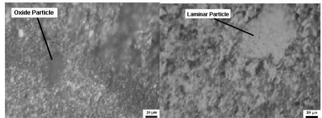
Figure 9. Wear particles generated in the fourth week of the first experiment. The first photo is of the inner ring of RPD observed with transmitted and reflected light. The second photo is of the outer ring with the same lights.
