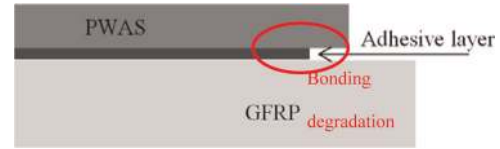
Figure 8. Bonding degradation model.
