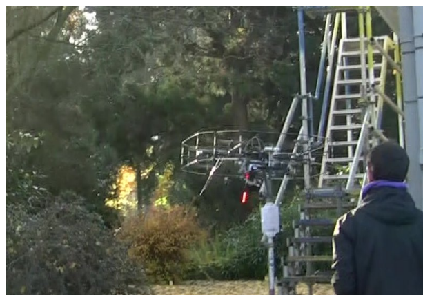
Figure 1: Our local obstacle avoidance algorithm acts as a safety measure between control inputs given by a planning layer or a human pilot remotely controlling the robot. This ensures safe operation in challenging situations, e. g., narrow passageways.
