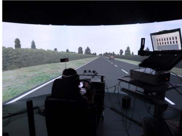
Fig 1. NITES 2 driving simulator and fNIRS apparatus. Photograph of the experimental setup. The participant is driving along the single carriageway road used in this experiment. The fNIRS computer is shown on the right; during the experiment this was positioned behind the participant out of their field of view.
