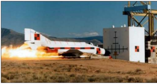
Fig.5: Full-scale impact test of a Phantom F4 fighter (Sugano et al., 1993-1)
