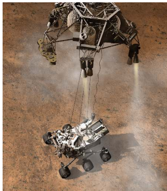
Figure 1. Artist’s concept of novel Sky Crane system used to land Curiosity . Image Credit: NASA/JPL-Caltech.
