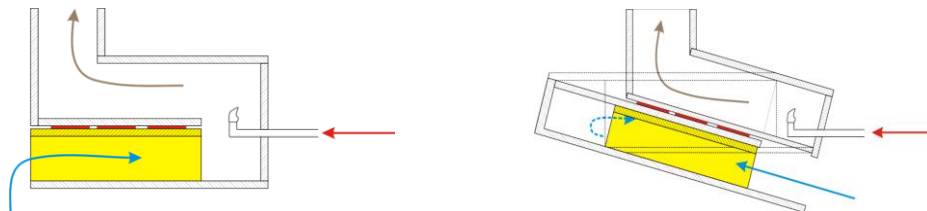
Figure 2. A possible counter-current (left) and co-current (right) flow arrangement (for color image see journal web site)
