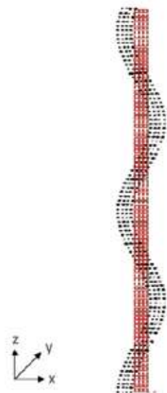
Figure 10. Proposed IBITT tunnel deformation during a M=7 earthquake, due to connected prefab units
