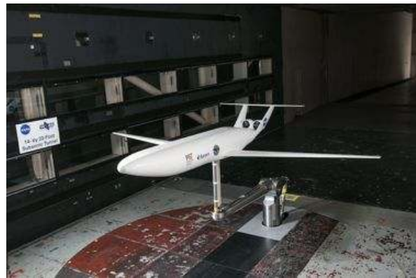
Figure 1. D8 model in BLI integrated configuration in NASA Langley’s 14×22 wind tunnel during the August–September 2013 experiments (photo credit NASA/George Homich).
