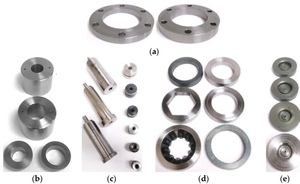
Figure 11. Experimental setup parts: (a) Support rings; (b) guiding zone inserts; (c) punch assemblies; (d) die inserts; and (e) bottom sealing inserts.
