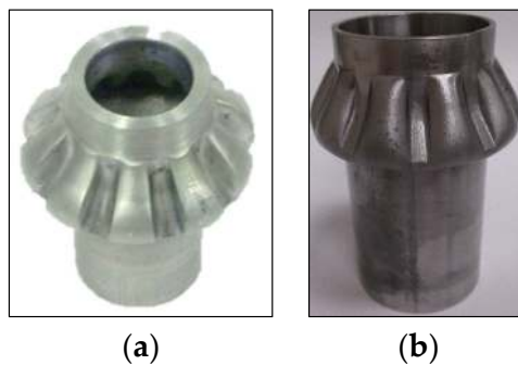
Figure 16. Bevel gear: AL6061(a) and SS304 (b).
