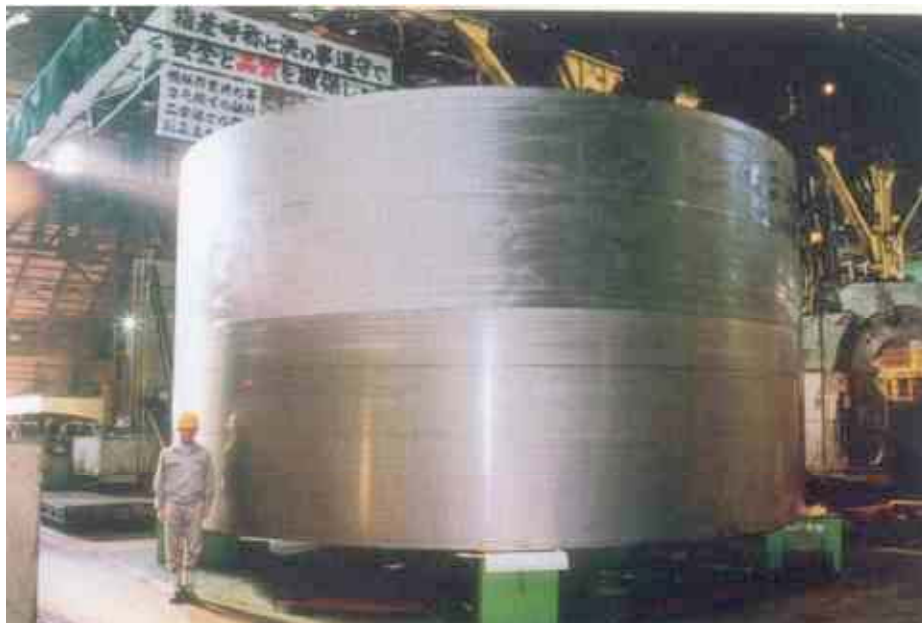
Figure 3.57. Large diameter ring forgings manufactured by Japan Steel Works [Nanstad, 2004].
