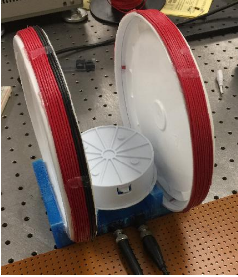
Fig. 8 (Left) Helmholtz coil constructed from bucket lids using 3D printed base: N = 20 , R = 10.55 cm. Left BNC port attaches to input and output contacts of coils and right BNC port measures voltage across a 2.1 \Omega resistor in series with the coils. (Right) Plot of calibration for pair of Bdot probes used in third design iteration.
