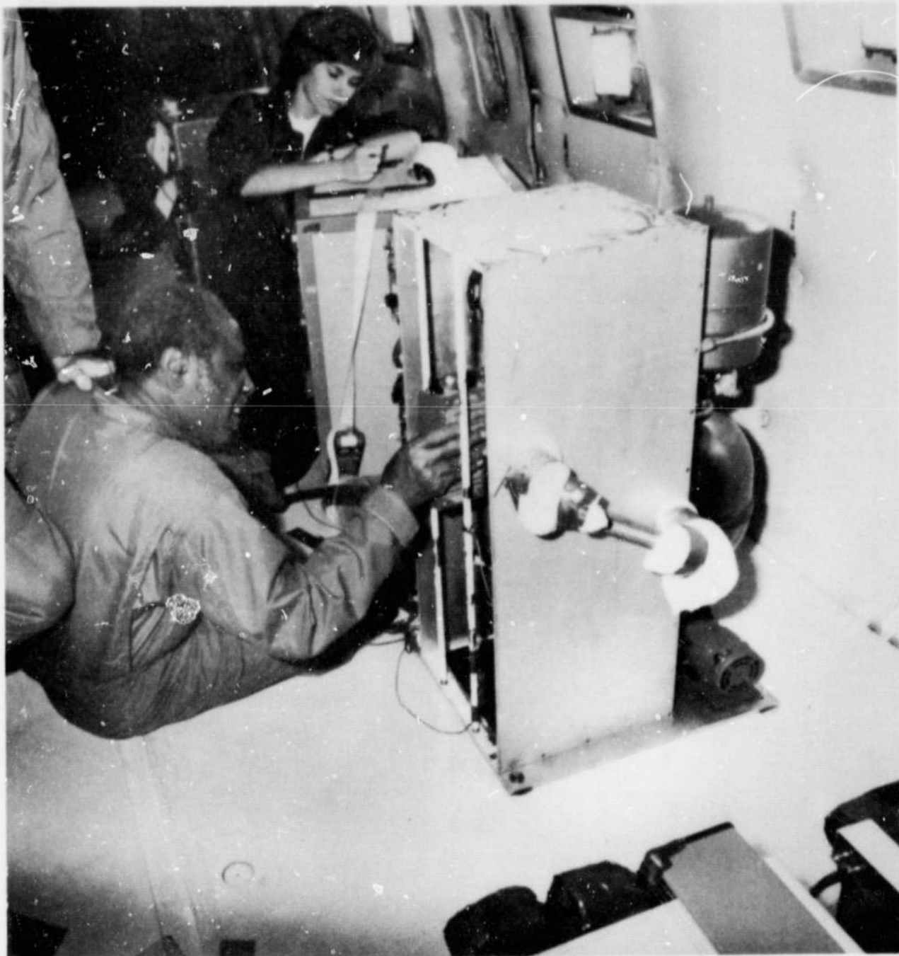
Figure 7. Directional solidification system being operated during the 9-22-82 KC-135 flight. (MSFC personnel Robert Shurney is measuring furnace RPM, and Wendy Alter is taking data.)
