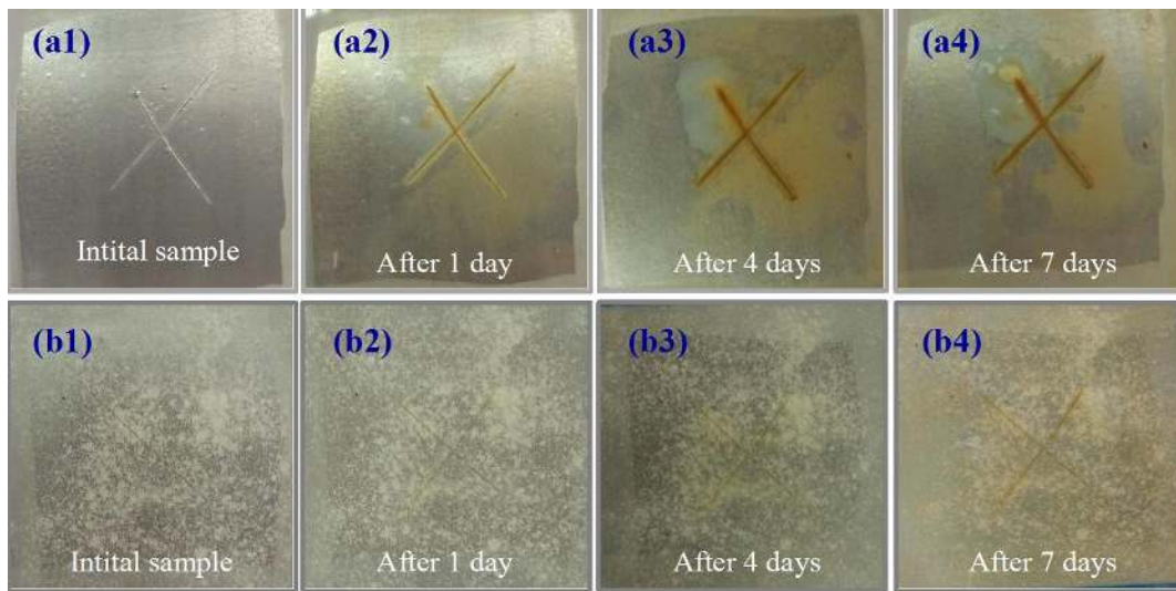
Figure 6 Optical photographs of corrosion protection of steel plates: (a1-a4) pure control epoxy scratched coating with immersion time of 0, 1, 4, 7 days, (b1-b4) self-healing epoxy scratched coating by incorporating 10 wt% microcapsules with immersion time of 0, 1, 4, 7 days
