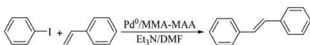
Scheme 2 Poly(methyl methacrylate- ran -12.1 mol% methacrylic acid) (MMA-12.1% MAA) supported \text{Pd}^0 catalyzed the Heck reaction between iodobenzene and styrene to produce trans -stilbene.
