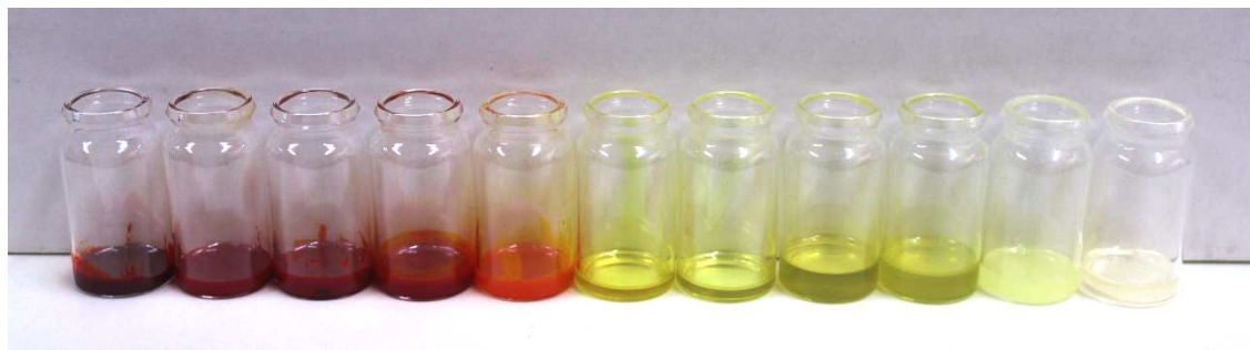
Figure 1. [\text{C}_4\text{C}_1\text{Im}]^+ based halobismuthate ionic liquids with different anions (from left to right): [\text{BiI}_3\text{Br}]^- , [\text{BiI}_3\text{Cl}]^- , [\text{BiBr}_2\text{I}_2]^- , [\text{BiCl}_2\text{I}_2]^- , [\text{BiBr}_2\text{ClI}]^- , [\text{BiBr}_4]^- , [\text{BiBr}_3\text{Cl}]^- , [\text{BiBr}_3\text{Cl}]^-_{0.5}[\text{NTf}_2]^-_{0.5} , [\text{BiBr}_2\text{Cl}_2]^- , [\text{BiBrCl}_3]^- , [\text{BiCl}_4]^- .
