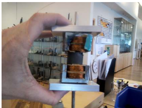
Figure 4. The magnetic spring element used for the prototype.
