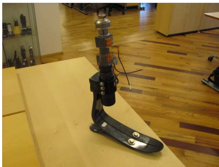
Figure 5. A prototype of a prosthetic foot with an MRE spring element.
