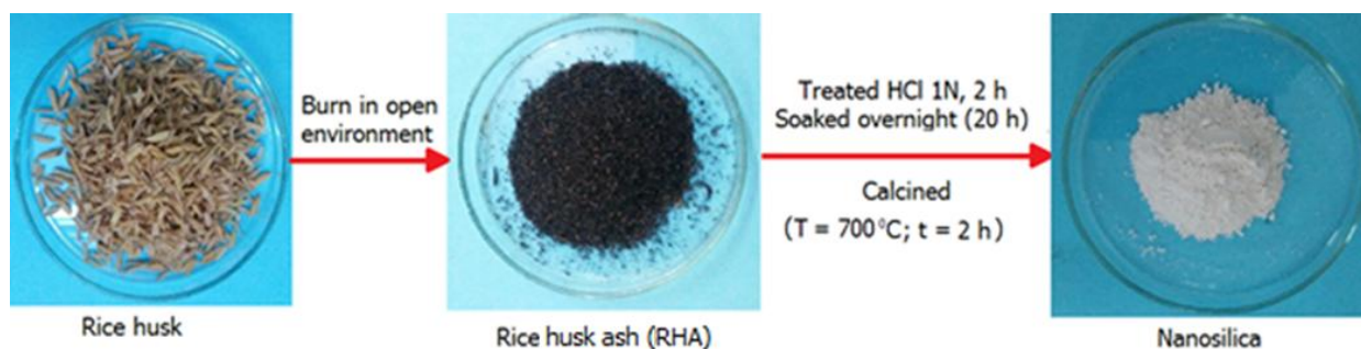
Figure 1: Schematic illustration of the synthesis mechanism for nanosilica powder from rice husk ash
