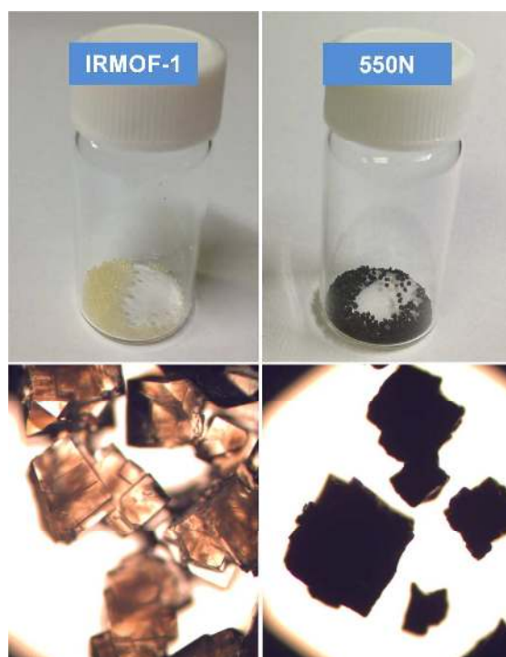
Figure S3. Photographs (top) and optical micrographs (bottom) of the IRMOF-1 and 550N.
