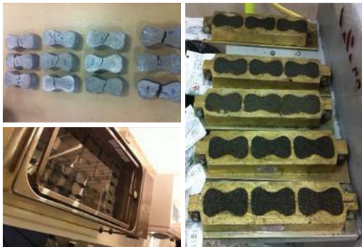
FIGURE 6: Samples and sample molds used for tensile strength test ASTM C307.
