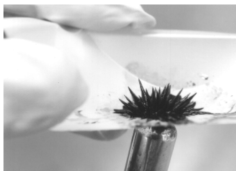
Figure 6. A side view of the spiking effect of an aqueous-based ferrofluid in the presence of a cow magnet, which is placed underneath a weighing boat.
