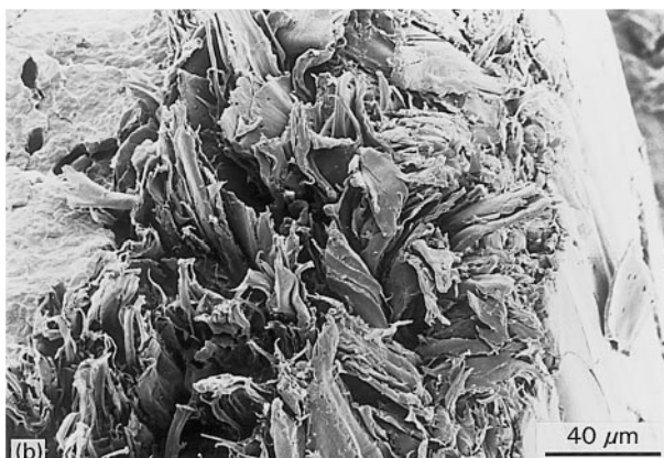
Fig. 5: Collapse in cellular structure of wheat straw (a) before and (b) after melt processing with polypropylene
