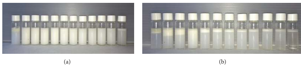
FIGURE 3: Set of emulsions prepared with C. guianensis oil and sorbitan monooleate/polysorbate 80 at different ratios (from left to right: HLB 4.3; 5; 6; 7; 8; 9; 10; 11; 12; 13; 14; and 15). (a) represents macroscopical characteristic of the emulsions on the day of preparation. (b) represents macroscopical characteristic of the emulsions after 7 days of storage (25°C).
