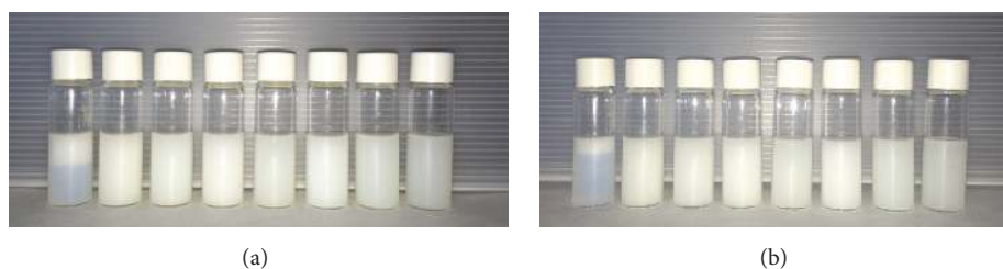
FIGURE 4: Set of emulsions prepared with C. guianensis oil and single surfactants or blends as follows (from left to right): polysorbate 81 (HLB = 10), polysorbate 85 (HLB = 11), polysorbate 80/polysorbate 85 (HLB = 11.5), polysorbate 20/polysorbate 81 (HLB = 12), polysorbate 20/polysorbate 85 (HLB = 12), polysorbate 80/polysorbate 81 (HLB = 12), polysorbate 80/polysorbate 85 (HLB = 12), and polysorbate 80/polysorbate 85 (HLB = 12.5). (a) represents macroscopical characteristic of the emulsions on the day of preparation. (b) represents macroscopical characteristic of the emulsions after 7 days of storage (25°C).
