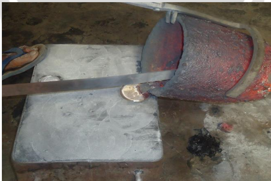
Fig 7: Pouring of molten Al into mould
