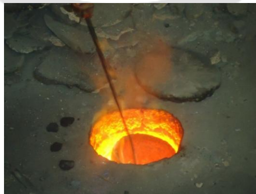
Fig 3: Melting of Al 6061 in pit furnace
