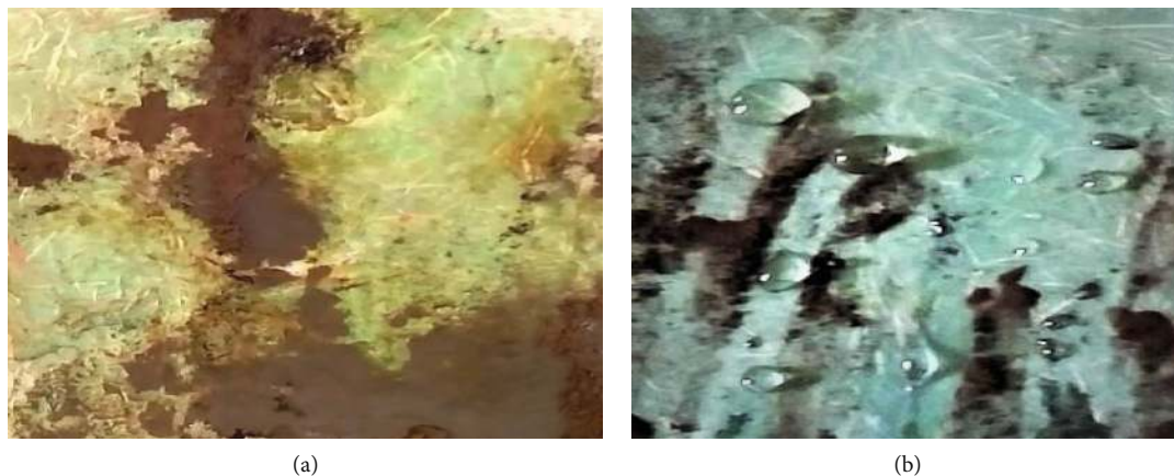
FIGURE 14: Self-cleaning properties of composite material (a) before surface modification and (b) after surface modification.
