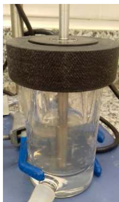
Figure 7. Bench reactor equipped with an impeller without blades used in the production of cyclodextrins from pre-hydrolyzed cassava starch using CGTase CLEA as biocatalyst.
