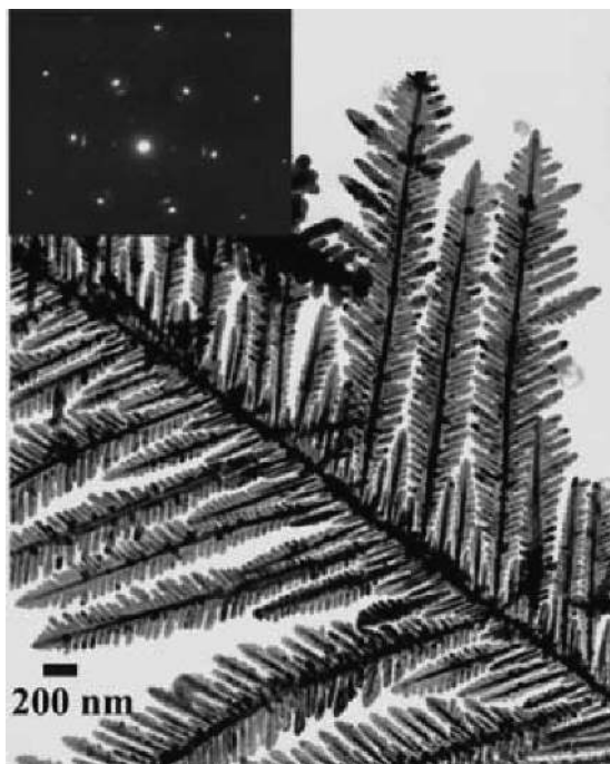
Figure 1. Typical HRTEM image of the dendritic Cu nanostructure. The sample was obtained at a potential of -1.0 V with an electrolysis time of 600 s in a 10-mL aqueous solution containing \text{CuCl}_2 (0.1 M) and \text{Na}_2\text{SO}_4 (0.1 M).
